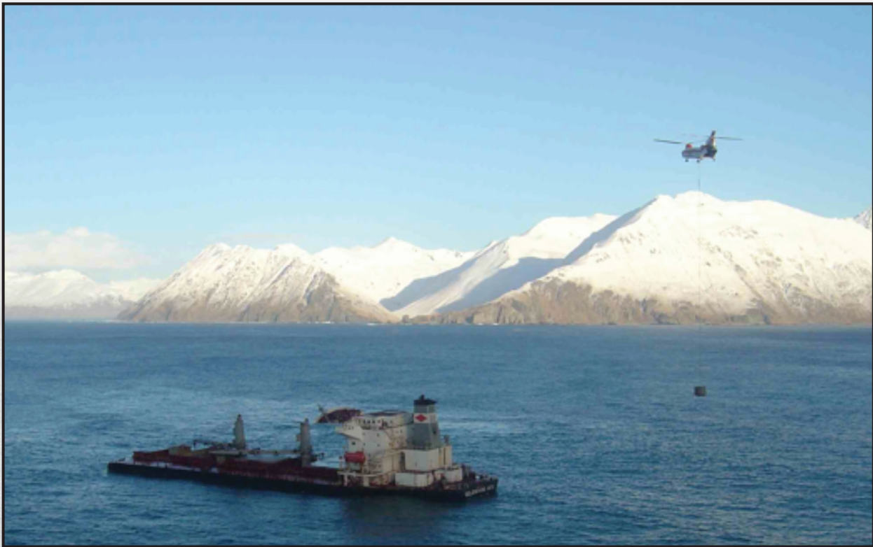
Figure 8. Lightering the Selendang Ayu using heavy lift helicopter and tanks. Used with permission. Photo credit: Unified Command
