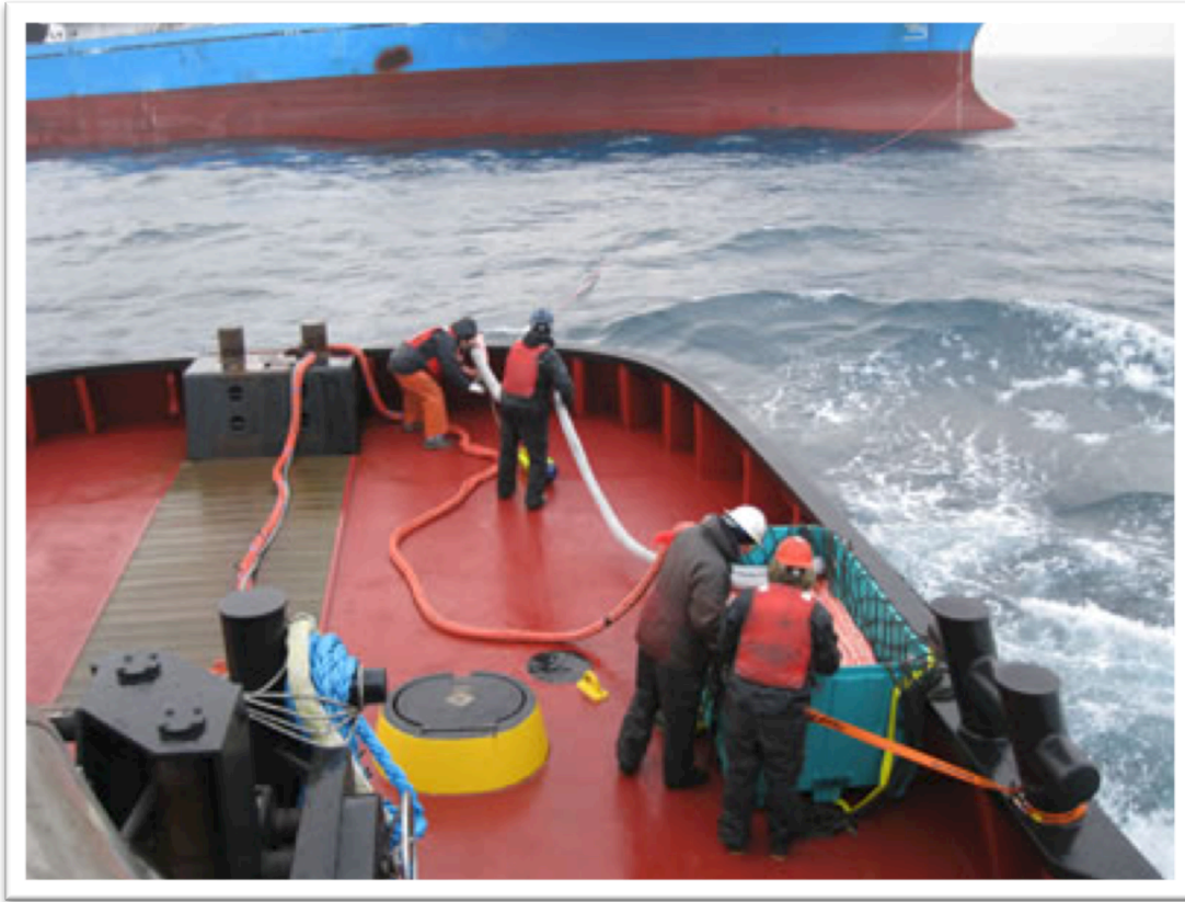
Figure 11. ETS deployment being prepared during October 2012 exercise in Unalaska Bay
