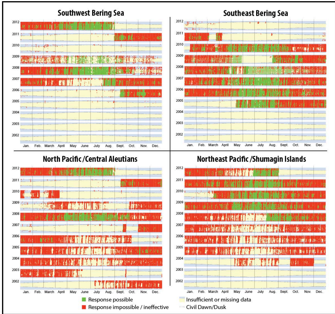
Figure A-6 Distribution of RGI at each buoy station for DISPERSANT APPLICATION FROM VESSEL
