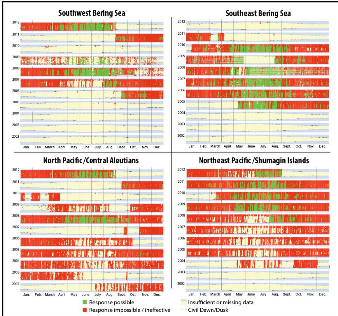
Figure A-3 Distribution of RGI at each buoy station for OPEN-WATER MECHANICAL RECOVERY
